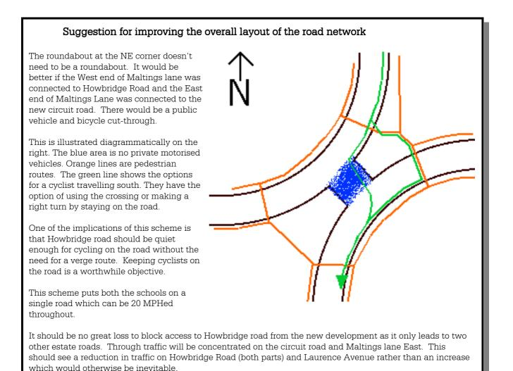
This layout and network would be safer than a roundabout for vulnerable road users.
